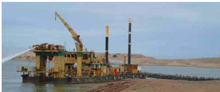
The Beach Comber Dredge in action, digging up sand for beach accretion.
