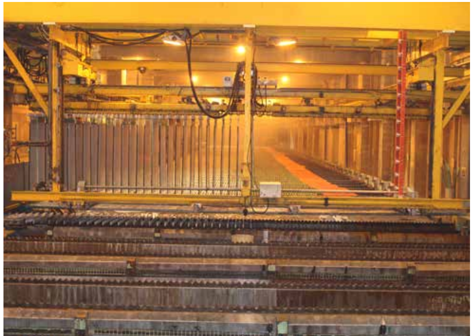
Electrowinning process at the Skorpion Zinc Refinery Plant
